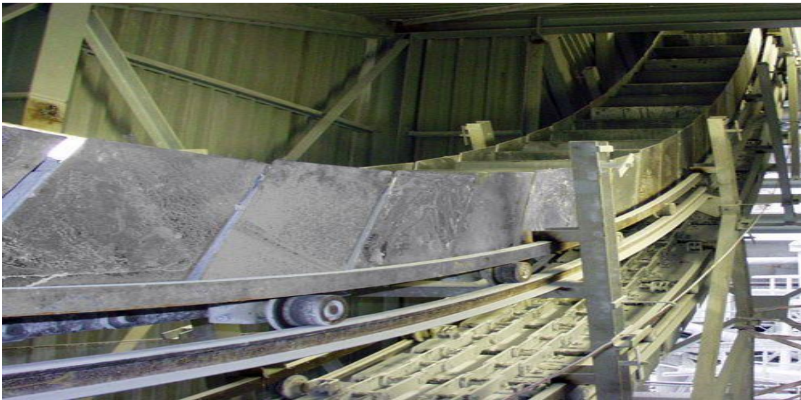
Figure 0-4 TC - Box conveyors [4]
